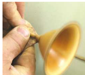
▲ Pic.11 When sanding the stem support the work like this; work through the grits, making sure the abrasive cannot wrap itself around the work
